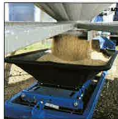
Collapsible intake flood fills the belt.
