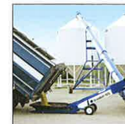
15- or 20-inch transfers available with hydraulic drive.
